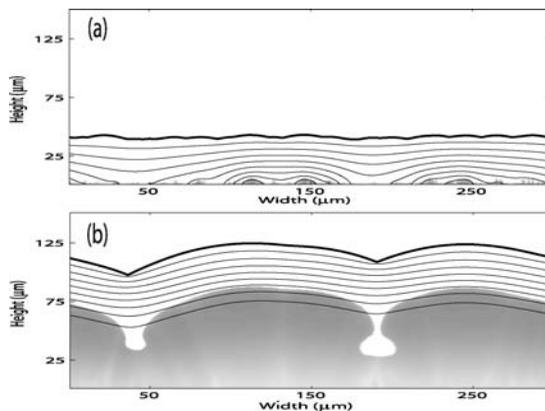
**Fig. 6** Time evolution of sparsely inoculated initial condition at times  $t = 0$  (a) and  $t = 15.5$  (b). *Gray color* represents active biomass. *Contour lines* show oxygen profiles in the biomass and liquid. The *thick black line* is the boundary  $\Gamma_{H_b}$ .
