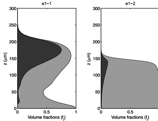
**Fig. 5** Averaged volume fraction of *e1-1* and *e1-2* by (21) at times  $t = 41$  and  $t = 32$  days, respectively. *Black area* represents active biomass and *light gray* inert material.
