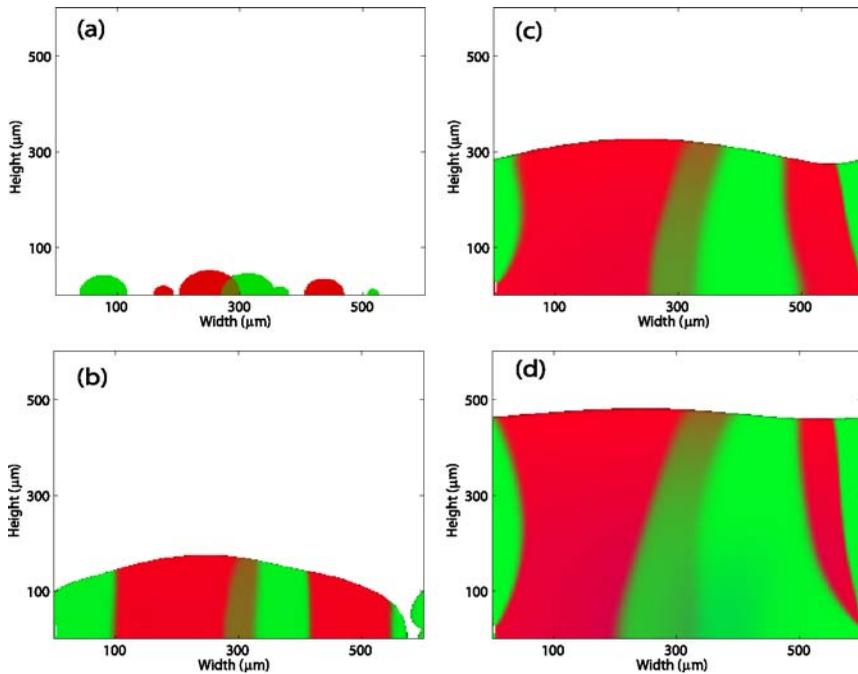
**Fig. 8** Two-dimensional simulation denoted  $e2-2$  for the biofilm system described in example 2 with an initial condition described by joint and disjoint colonies of different species. Illustrations use the RGB channels where *red* represents the heterotrophs, *green* the autotrophs, and *blue* the inert biomass. Time evolution through *top left* (a)  $t = 0$ , *bottom left* (b)  $t = 3.5$  days, *top right* (c)  $t = 5.9$  days, and *bottom right* (d)  $t = 7.8$  days.
