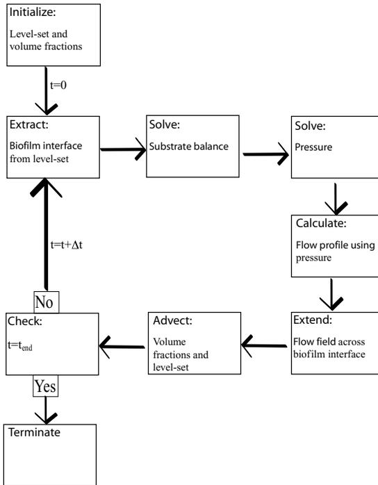
**Fig. 3** Flowchart of the computational scheme.
