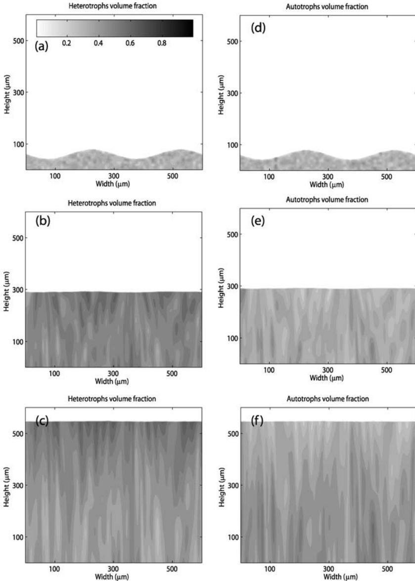
**Fig. 7** Two-dimensional simulation denoted  $e2-I$ , for the biofilm system described in example 2 with an inhomogeneous initial condition. Volume fractions of heterotrophs and autotrophs are illustrated by filled isocontours. The left column (a), (b) and (c) shows the heterotrophs and the right column (d), (e) and (f) shows the autotrophs. Time evolution from *top* to *bottom*: (a) and (d) at  $t = 0$ , (b), and (e) at  $t = 2.1$  days, (c) and (f) at  $t = 3.1$  days.
