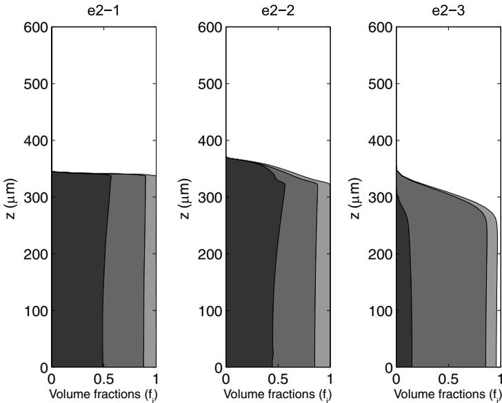
**Fig. 10** Averaged volume fraction of  $e2-1$ ,  $e2-2$ , and  $e2-3$  using (21), at times  $t = 2.4$ ,  $t = 6.4$ , and  $t = 5.2$  days. *Black area* represents the heterotrophs, *dark gray* the autotrophs, and *light gray* the inert materials.
