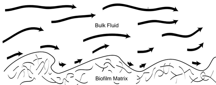
Figure 2. Cartoon of a biofilm–bulk fluid system. Bulk fluid flow above the biofilm–bulk fluid interface provides a source of substrates for the biofilm as well as imparting mechanical stress. Individual entangled EPS polymer chains are depicted within the biofilm matrix [after Koerstgens *et al.* (2001)].
